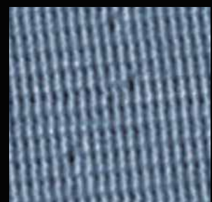
Single crystal calcite (CaCO 3 ) imaged in water with Cypher AFM, courtesy of Asylum Research
